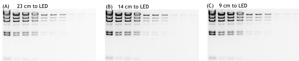
Figure 3. Epi-Blue LED excited SYBR Gold stained agarose gel in KETA ML with 0.2 seconds exposure time.
