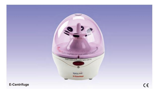
Small footprint desktop centrifuge is designed for quick spin down from the suspension. Supply with interchangeable angle rotor for 6 positions of 1.5 / 2.0ml tubes, and strip rotor for  $8 \times 2$  positions of 0.2ml PCR tubes. Optional adapter is available 0.4 / 0.5ml tubes, and interlock switch secures top lid suddenly opened.
