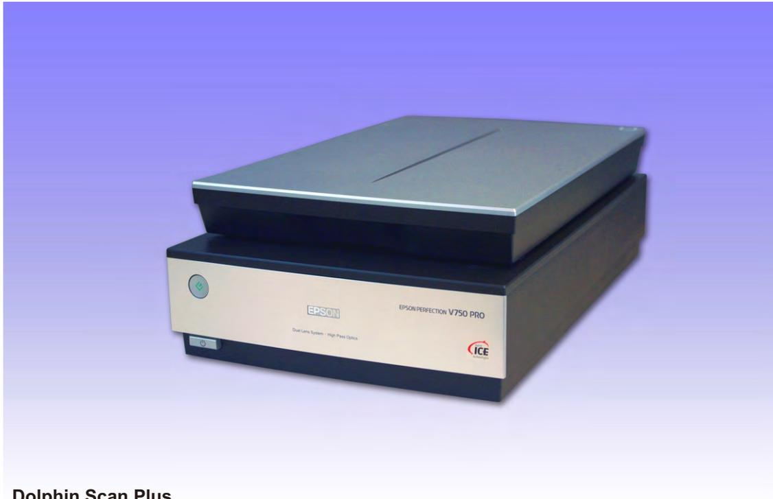
Dolphin-Scan Plus is a professional Scanner for 2-D Gel, SDS-PAGE, Western Blot, X-ray film serving for high resolution image catch. Both transparency and reflectance mode are applicable for whether the samples are dry or wet.
