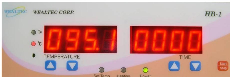
**Figure 3:** When the unit is warm enough, the “Heating” indicator will turn off. Press the Stop/Start-button to access the timer-settings. The time will be shown on the right display.
